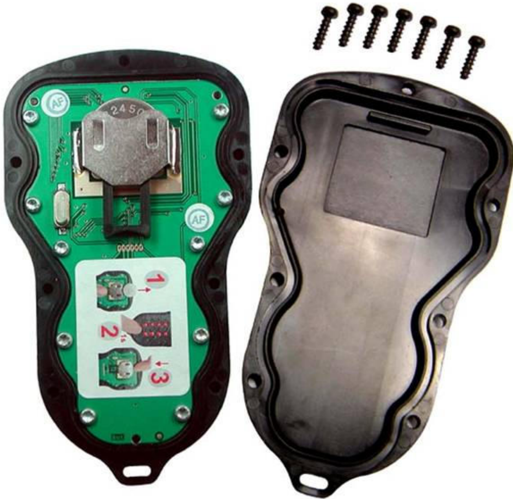
Operation to carry out when replacing the type CR2450 battery
