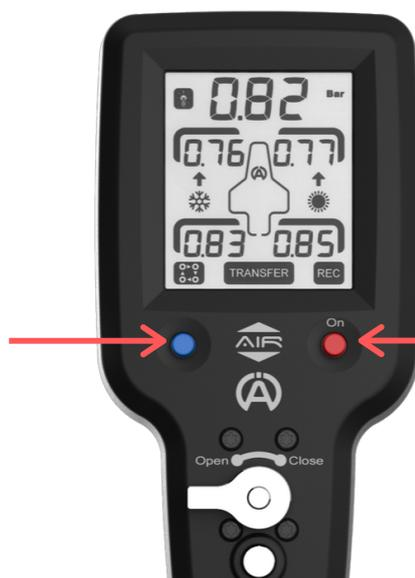
Transfer the pressure as hot tyre pressure
