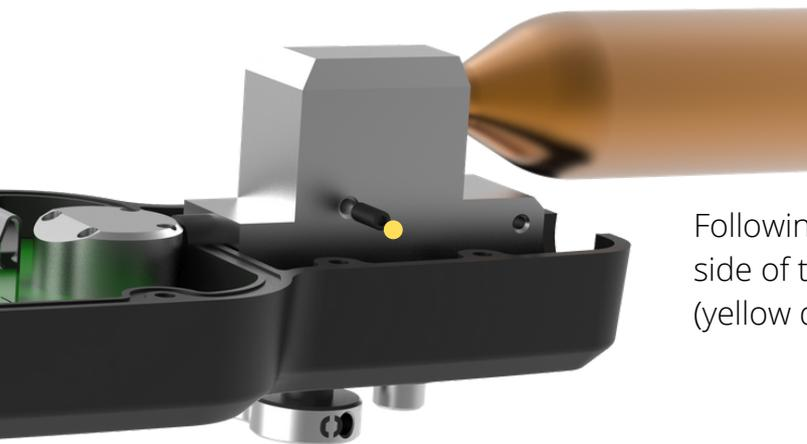
Following that step, unscrew the M3x8 screw on the side of the metallic part with a 1.5 mm Allen key (yellow dot on the image on the left)
